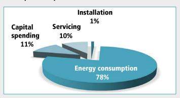
After 5 years of operation, the energy cost usually amounts to 78% of the total cost of a conventional compressor. The only way to reduce the overall cost is to reduce the cost of energy.
